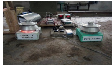
Fig.6: Experimental setup for performance tests using coating of aluminum sheet
