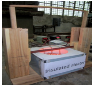
Fig.3: Experimental setup for temperature profile of insulated heater along radial and vertical direction
