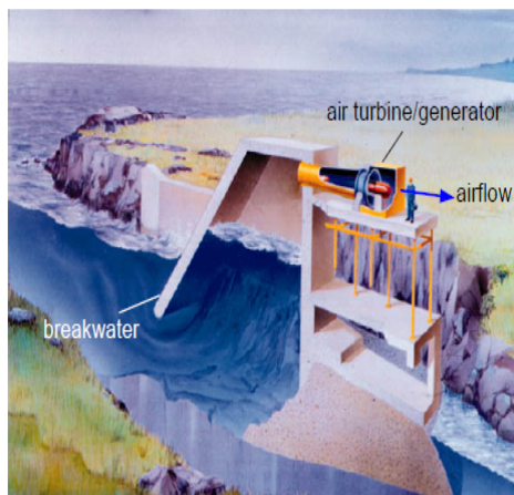
Fig. 2: Oscillating water column [15]
