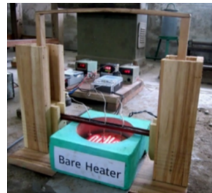
Fig.4: Experimental setup for temperature profile of bare heater along radial and vertical direction
