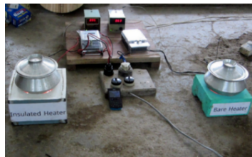
Fig.5: Experimental setup for performance tests using glass wool insulation and white cement
