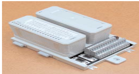
Fig 4: Turbine control module
