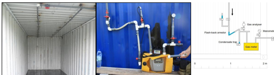
Figure 3: Percolate sprinkling, gas measurement bench, scheme of gas measurement (left to right)
