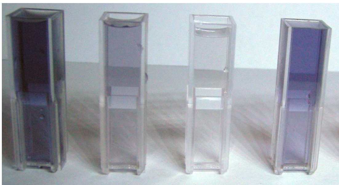
Figure 3: Use of fly as at a 5% dose of the total WW (left to right reads raw WW and colour removed from WW using Fly Ash#1, Fly Ash #2 and Fly Ash #3 respectively)
