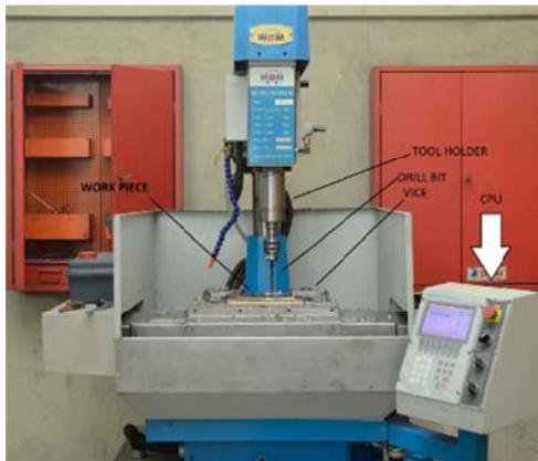
Fig. 2. Photograph of the CNC drilling machine
