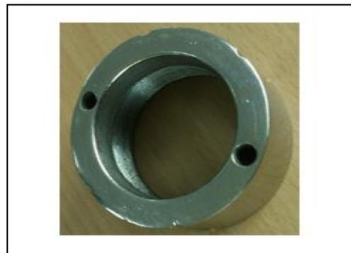
Fig. 2. Clamp sleeve spare part of crimping machine.
