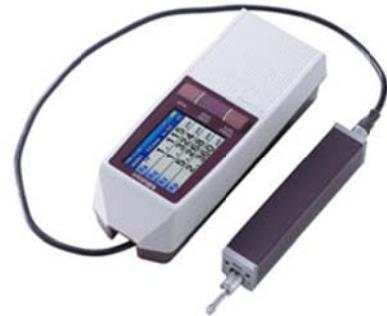
Fig. 6. Mitutoyo Surftest SJ-210 contact profilometer
