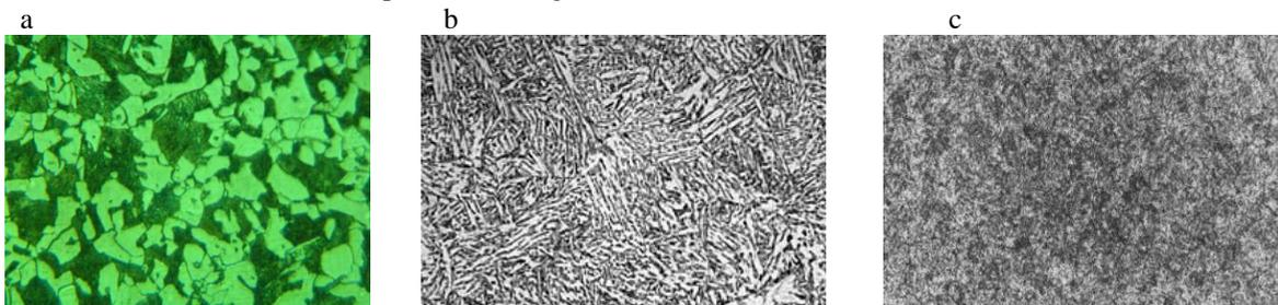
Fig. 6: Microstructure of low carbon steel (a) before heat treatment (b) after heat treatment (oil quenched) (c) after heat treatment (water quenched). Ethced with 2% Nital (Magnification 400x)
