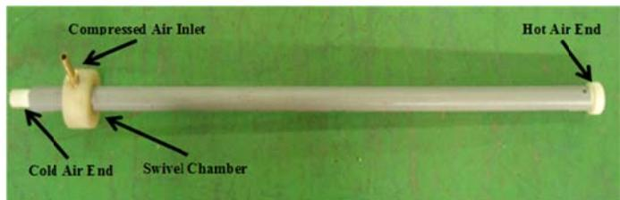
Fig. 3. Photograph of the developed Vortex tube
