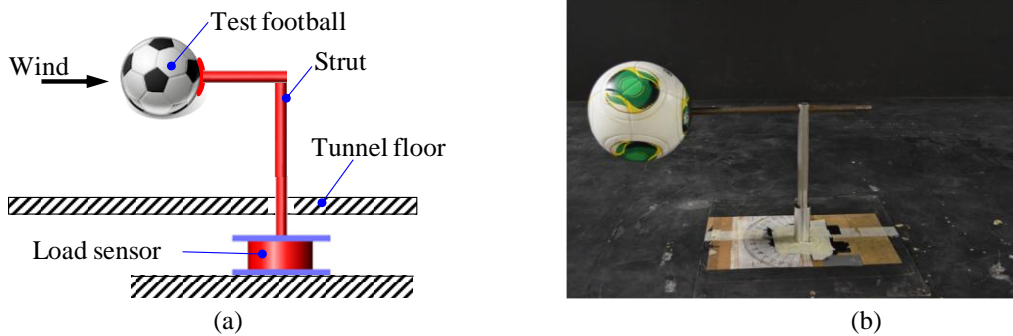
Fig. 2. (a) schematic of the experimental setup; (b) setup inside RMIT Industrial Wind Tunnel.
