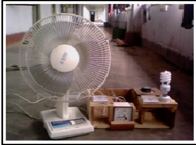
Figure 8: Measurement of power factor with inductive load.
