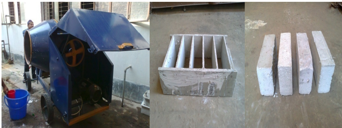
Fig. 1. Mixing machine, curing aluminum blocks and RHA bricks
