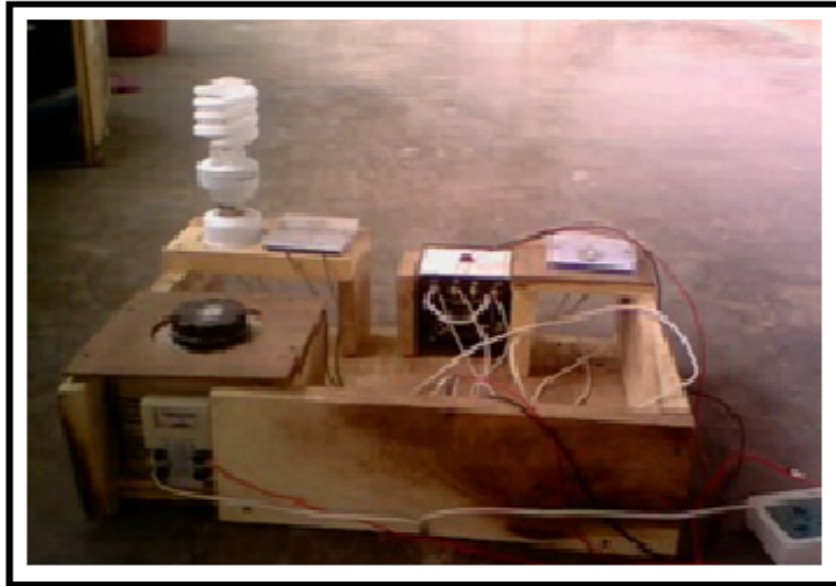
Figure6: Measurement of power factor with capacitor.
