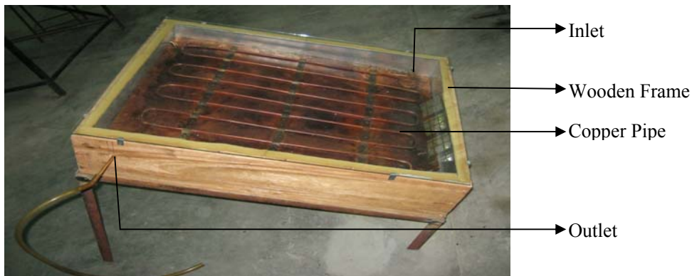
Fig.3 Photograph of our constructed solar collector
