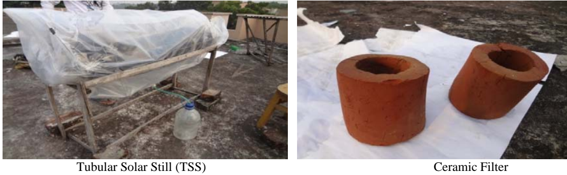
Fig.2. Structural components of a TSS-SF unit
