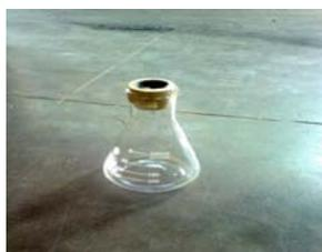
Fig.6: The airtight gas jar
