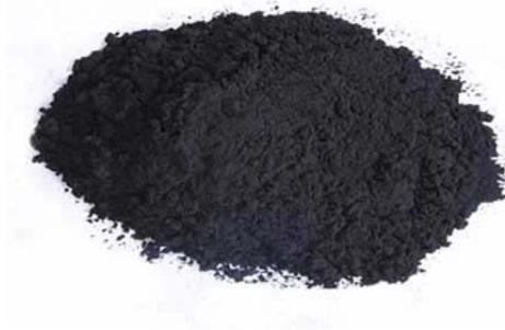
**Fig.1:** Activated powder carbon
