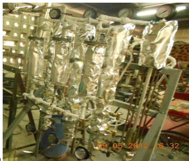
Fig. 4. Micro Scale Multi Effect Distillation (MSMED) Unit (a) before insulation (b) after Insulation.
