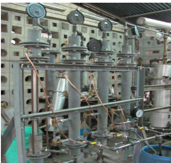
Fig. 4. Micro Scale Multi Effect Distillation (MSMED) Unit (a) before insulation (b) after Insulation.
