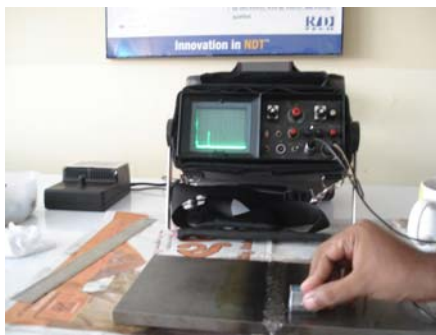
Fig 5. Observation of crack signal in the welded plate, A2 under ultrasonic testing.
