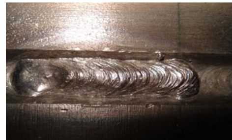
Fig 2. Photograph of the cracked welded plate (Specimen A1).
