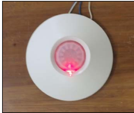
Fig 3. Motion detector mounted on the wall
