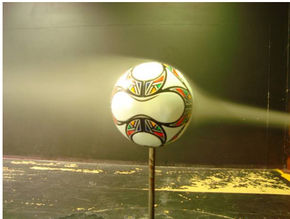
Fig 6. Airflow structure around a 14 panels football
