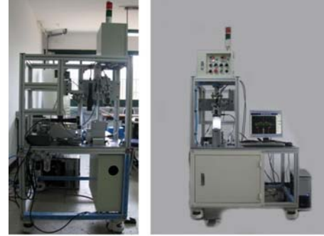
Fig 7. Implemented computer vision-based inspection system
