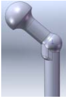
Fig. 4a. FE side view model of human femur.
