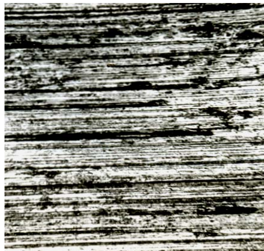
Fig 6. Wear pattern on steel counter body used for as-received nodular cast iron sample.
