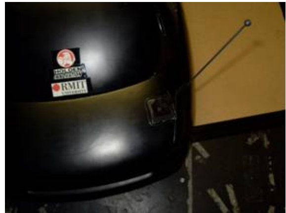
Fig 5. An antenna attached to the rear of the test vehicle
