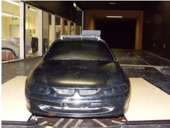
Fig 1. 25% Scale Model of GMH Commodore Vehicle (test vehicle) in the test section of RMIT Industrial Wind Tunnel
