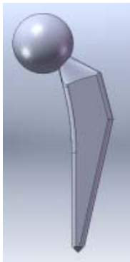
Fig. 5a. FE side view model of commercial total hip replacement
