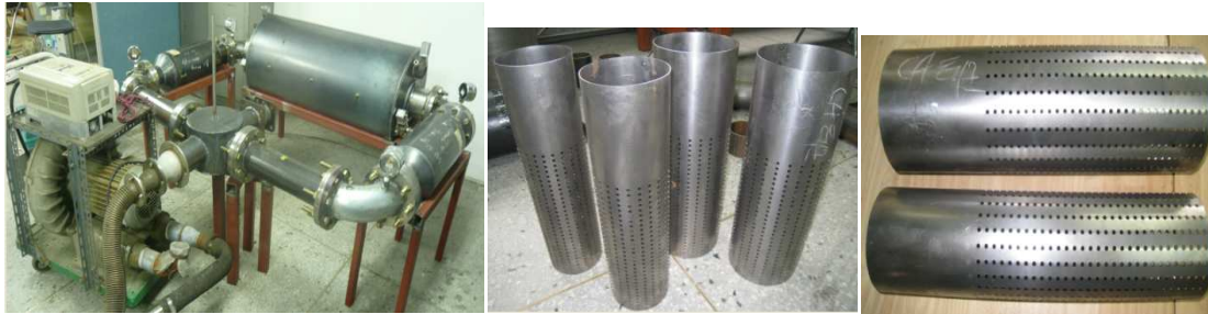
Fig:1 Layout of testing burner and testing air-distributors
