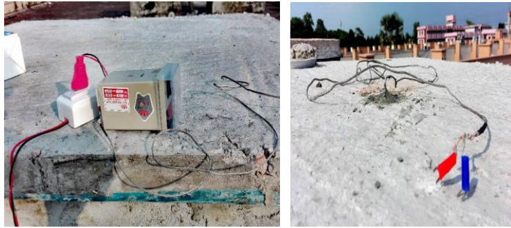
Figure 6: Thermocouple Setup on Slab
