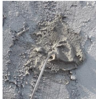
b) Thermocouple in slab
