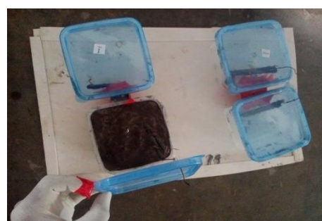
Fig. 3. Substrate placement in the anode chamber with electrodes
