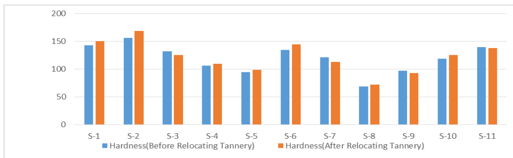
Figure 3: Comparison of Hardness level (mg/l) before and after the relocation of Hazaribagh tanneries.
