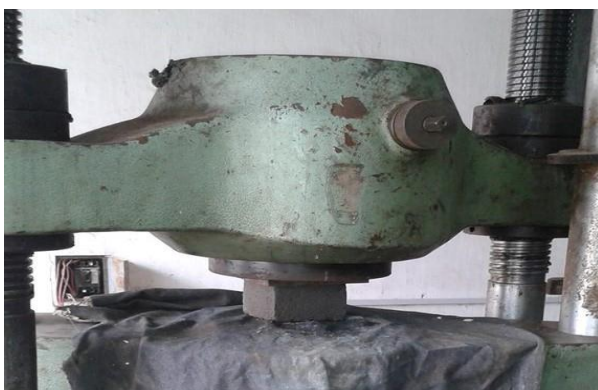
Fig.3: Testing sample in Universal testing machine
