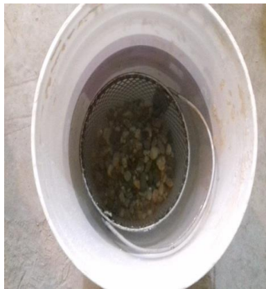
Fig. 4: Specific gravity and water absorption capacity test of CA.
