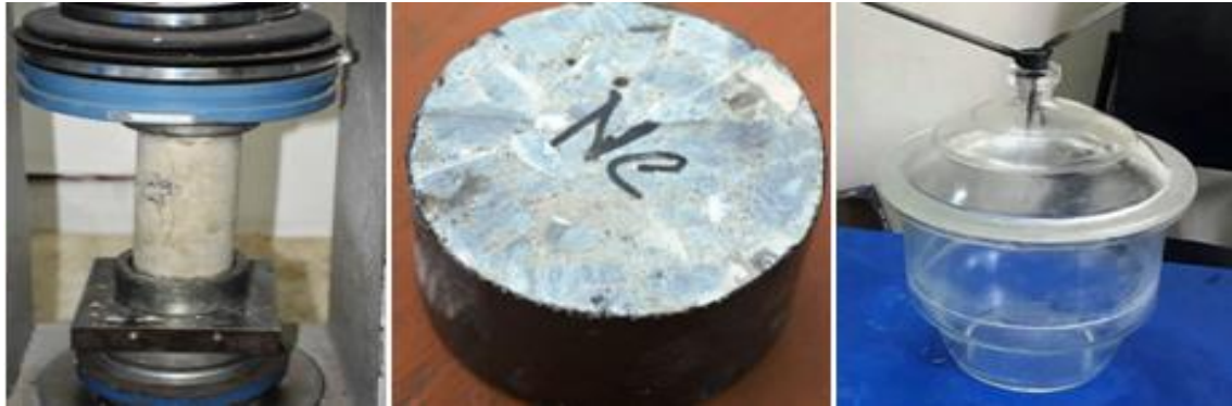
Fig.4: Compressive strength test Fig. 5: Epoxy coated specimen Fig.6: Vacuum Chamber
