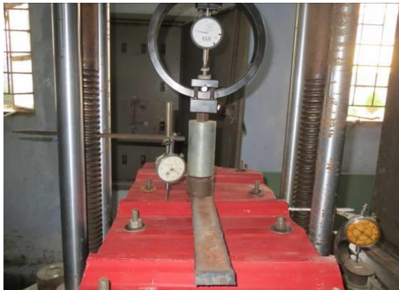
Figure 6: Test setup and failure of mode of web crippling test specimen
