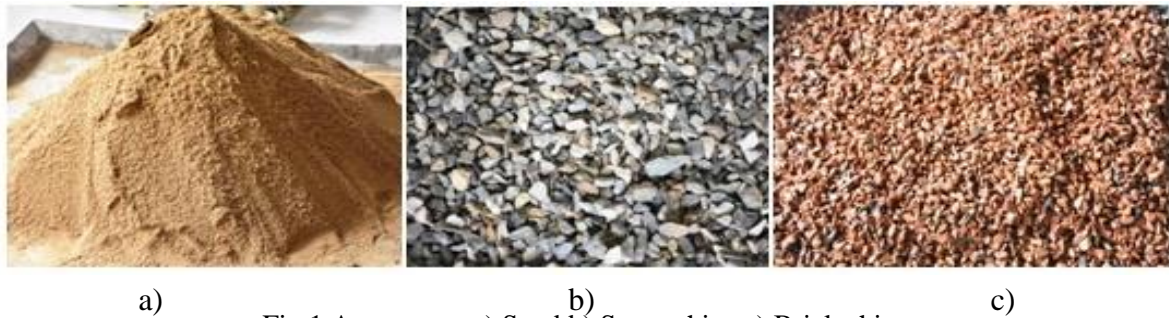
Fig.1 Aggregates a) Sand b) Stone chips c) Brick chips
