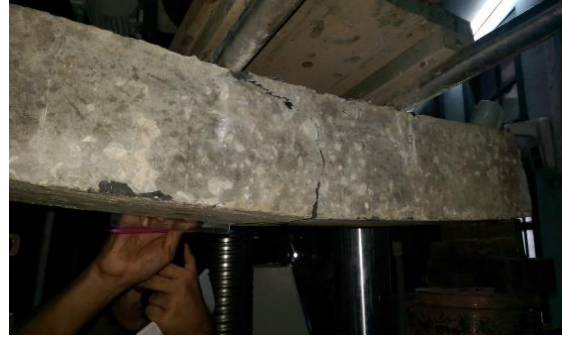
Fig. 3: Fracture of the beam during experiment
