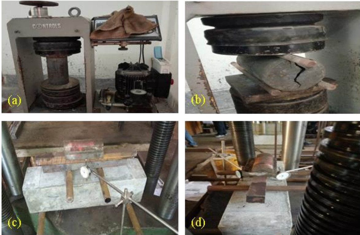
Figure 1. Experimental set up for (a) compressive strength test, (b) splitting tensile strength test, (c) flexural strength test, and (d) flexural toughness computation.
