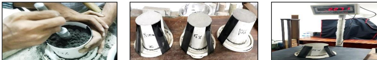
Fig. 1: Sample placing, tamping and measuring weight
