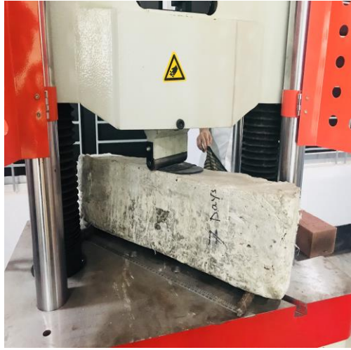
Fig. 11: Loading on RCC beam by UTM.
