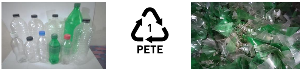
Fig. 1: Plastic particles cut down from PET bottles
