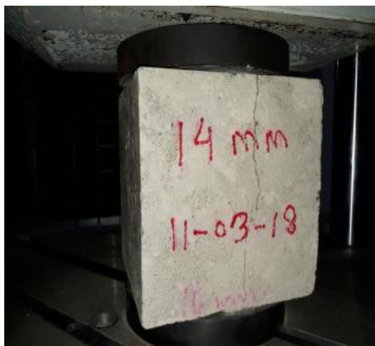
Fig. 8: Compressive strength test of concrete cube.
