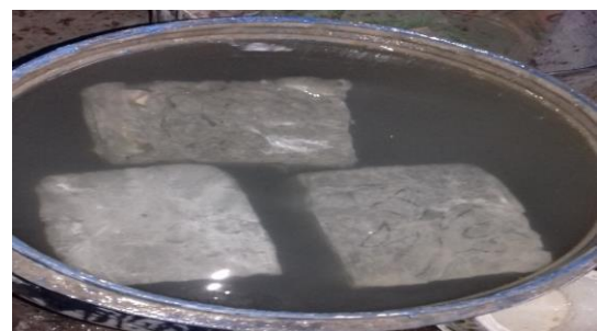
Fig. 10: RCC beam immersed under water for curing.
