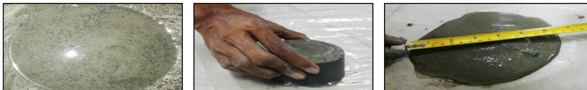
Fig. 2: Mortar paste, Molding & measuring diameter after demolding sample
