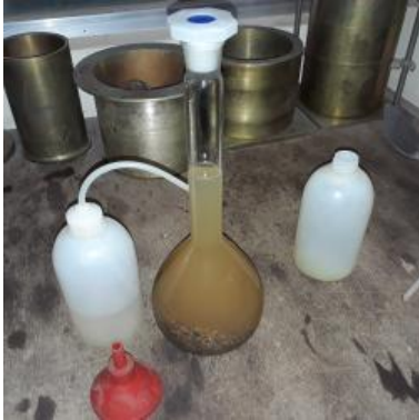
Fig. 2: Specific gravity and absorption capacity tests of FA.
