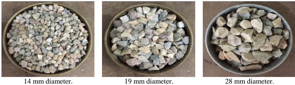
Fig. 1: Different sizes of coarse aggregates.
