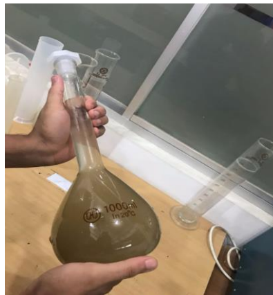
Fig. 2: Specific gravity and absorption capacity test for FA.
