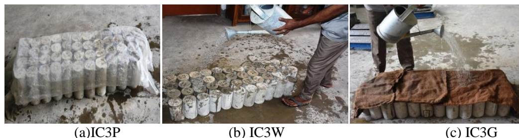
Fig. 3: IC samples exposed outside after 3 days curing under water
