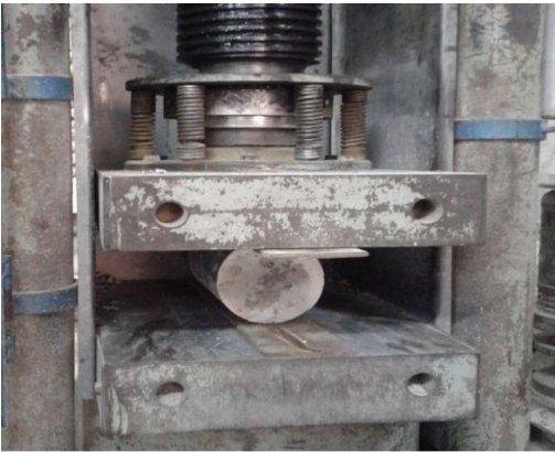
Figure 4. Test setup for splitting tensile strength
