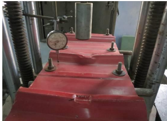
Figure 6: Test setup and failure of mode of web crippling test specimen
