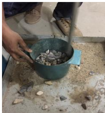
Fig. 5: Dry rodded unit weight test of CA.
