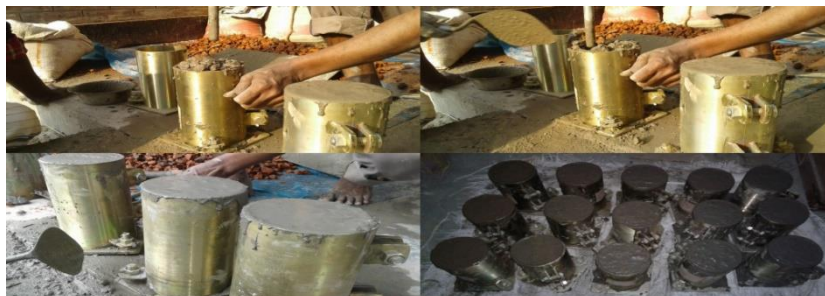
Fig. 3: Casting of Cylindrical Specimen.
