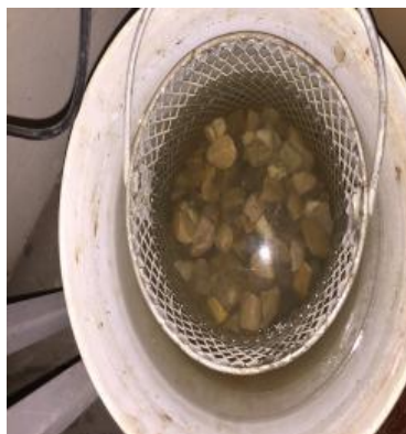
Fig. 4: Specific gravity and water absorption capacity tests of CA.
