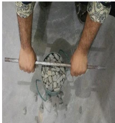
Fig. 5: Dry rodded unit weight test of CA.
