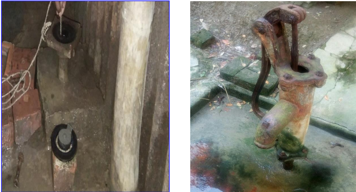
Figure-2: Determination of ground water level by thick wear in shallow tube well
