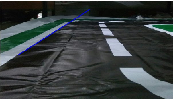
Fig. 9. After Hough transformation and drawing a Hough line
