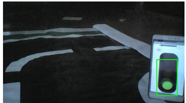
Fig. 6. Traffic light detection using Haar cascade classifier
