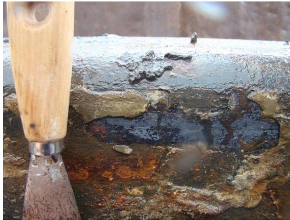
Figure 5. Crusts of mineral deposits formed by microbial communities on the surface of sheet pilings. Image courtesy of Michael Asanajef, Delft University of Technology
