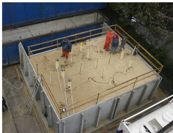
Figure 4. Pilot scale (100m<sup>3</sup>) bio-grouting experiment by van Paassen and colleagues.
