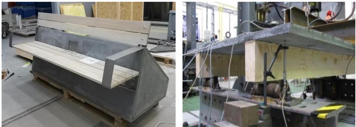
Fig 3 (a) prototype of solar bench CapaSitty made from UHPC at University Centre for Energy Efficient Buildings, CTU (photo T. Vlach), (b) hybrid timber-concrete floor structure - UHPC 30 mm thin slab is glued to glue laminated beams; testing at CTU Experimental Centre.
