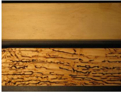
Fig. 5. Termite resistance of Acetylated wood (top) compared to non-treated wood of the same wood species (below).
