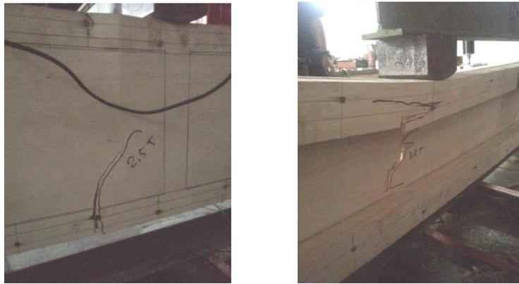
Fig 5. Failure mode of Box-section (left) and I-section (right) built-up joists under bending test
