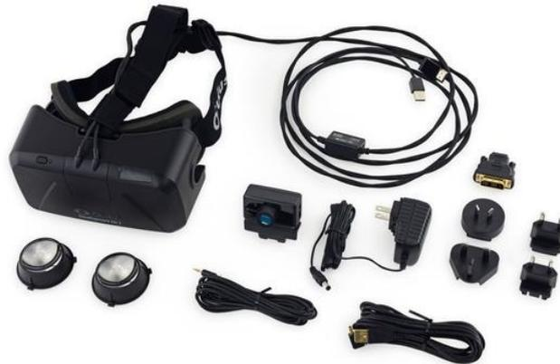
Fig. 7: Components of Oculus Rift DK2. (Source: <https://www.oculus.com>)
