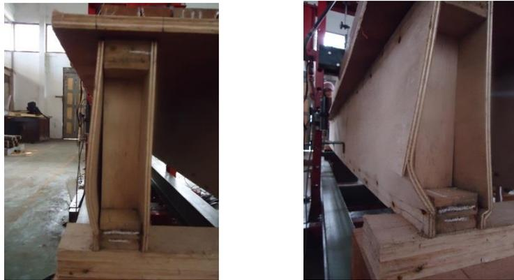
Fig 11. Photos of failure of the wood frame
