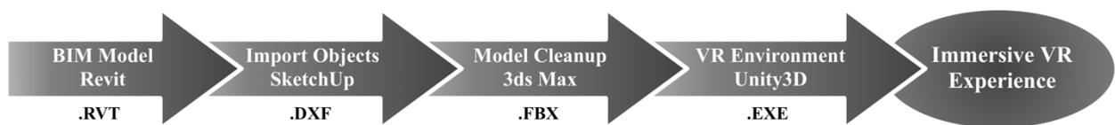
Fig. 8: Modeling workflow for developing a VR environment for safety training (Froehlich and Azhar, 2016)
