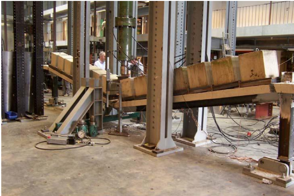
Figure 5: Test simulating column removal
