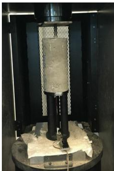
Figure 1: Fully assembled push out testing apparatus
