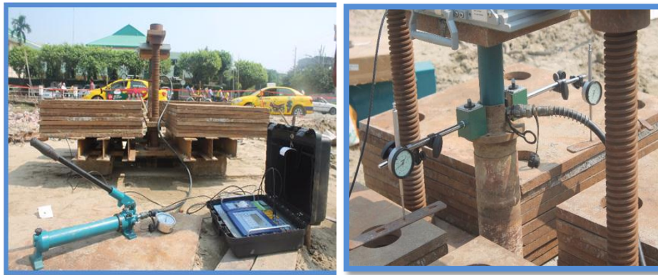
Figure 1: Photographs of SPLT setup: Overall arrangement (left) and dial gauges for measuring settlements (right)
