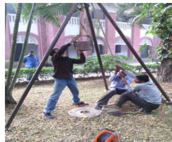
Figure 6: Using 140lb hammer as impulse source
