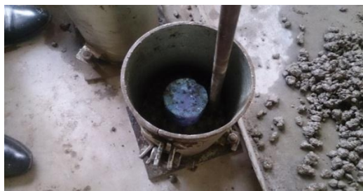
Figure 4: Placing the core at the center of cylinder
