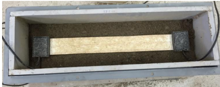
Figure 5: Placement of FRC sensor between soil layers in the calibration box
