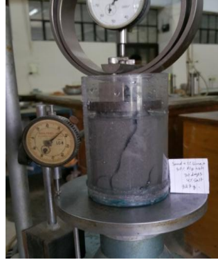
Figure 4: Submerged specimen for Unconfined Compression test.
