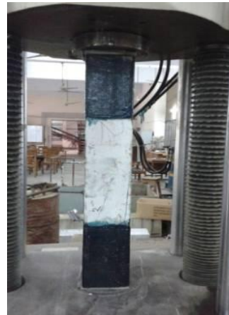
Figure 2: Typical X- section of FEC columns Figure 3: Experimental column test setup
