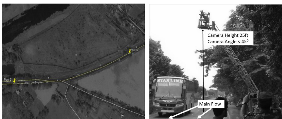
Figure 1: Test location map (courtesy: Google Map) (left), Details of camera setting at point 01 (right) (Data Collected on 26 October 2015; 0900 to 1200Hr)
