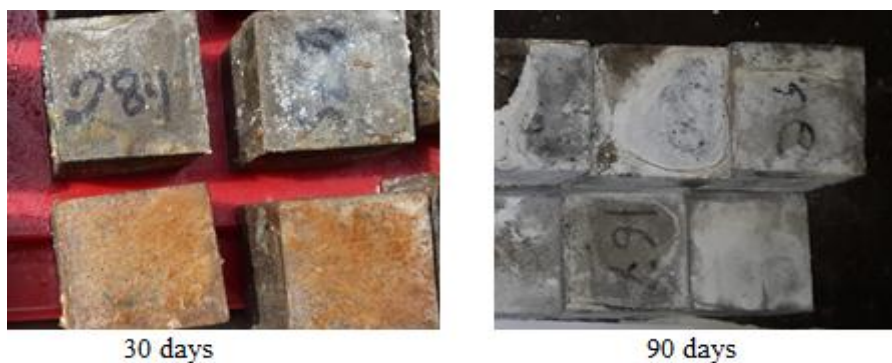
Figure 2: Specimens after exposure in 5% Hydrochloric acid solution
