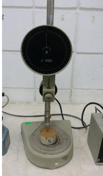
Figure 2: Measurement of soil liquid limit using cone penetrometer
