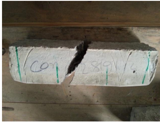
Figure.4. Flexural strength tested beam specimen
