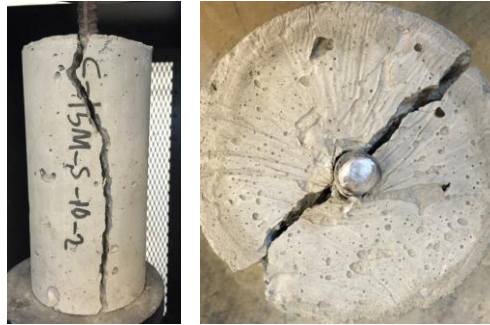
Figure 2: Failure of samples
