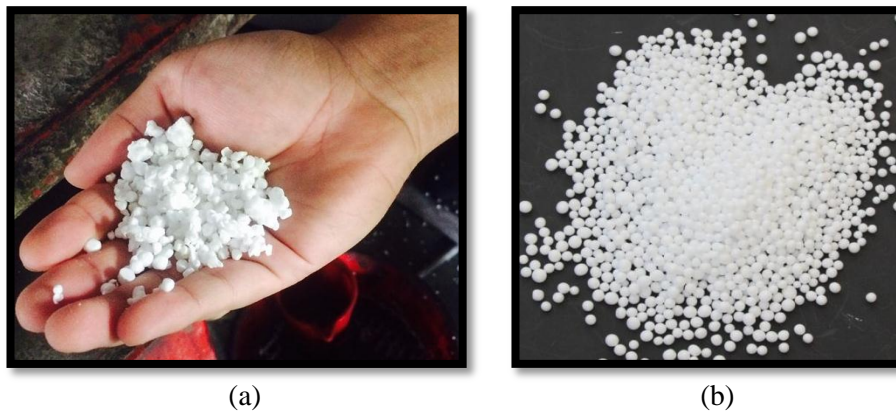
Figure 2: Polystyrene Bubble Sample (a) used in experiment [6] and (b) available in world-market.
