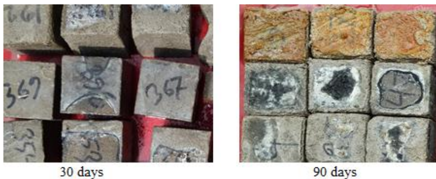
Figure 1: Specimens after exposure in 5% Sulfuric acid solution
