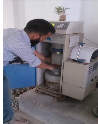
Figure 6: Crushing concrete in concrete testing machine
