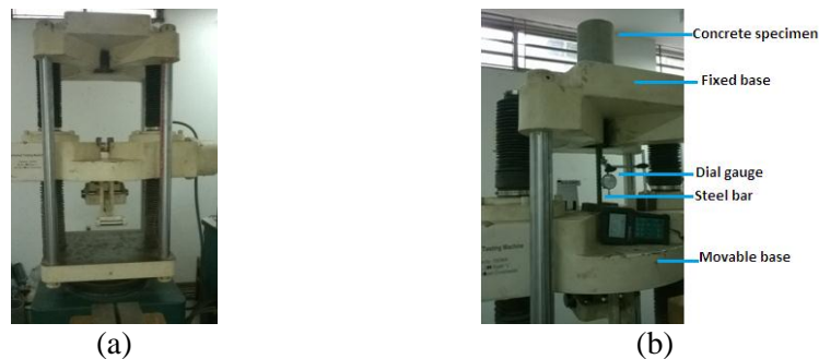
Figure 4: Test setup (a) UTM machine and (b) Sample specimen is placed at UTM
