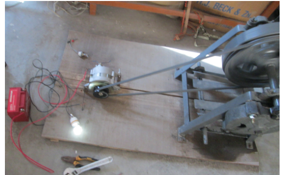
Fig. 1: Complete setup of the Pedal Generator system with DC generator, Storage and Light bulb
