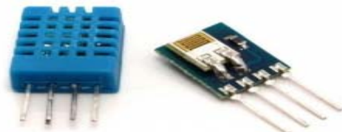
Figure 3. DHT11 Temperature and humidity sensor
