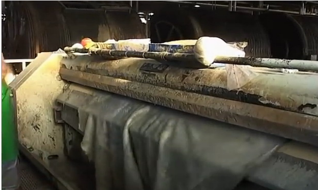
Fig.5 The fleshing machine is used to remove any fleshy matter from the leather and further used for biofuel production
