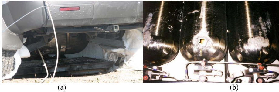
Fig. 1. (a) Car with burned cylinder, (b) Porosity due to multi pass and over pressure
