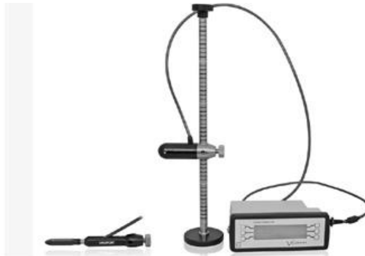
Figure 2: Experimental set up for Model 802 Water Flow Meter
