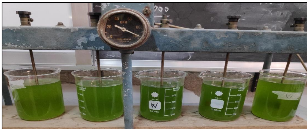
Figure 3 : Coagulation and flocculation process
