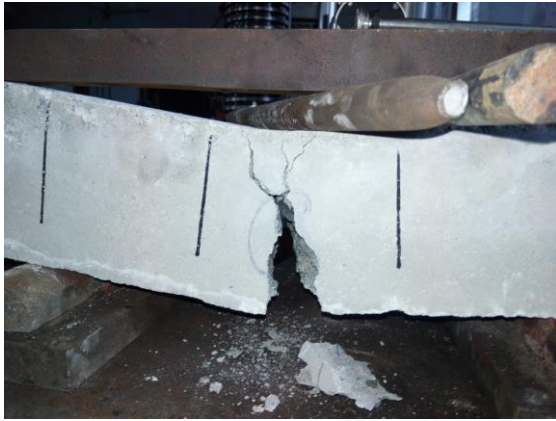
Figure 4: Failure of the beam in third-point loading test.
