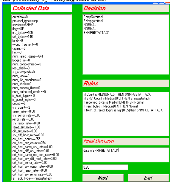
Fig. 14: NIDS for SNMPGETATTACK Summary all connection types have been given in Table 7.
