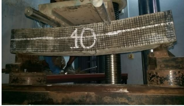
Fig. 2: Development of first crack in the beam
