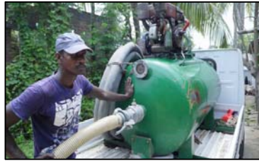
Vacutag provides septic tank and pit latrines emptying.
