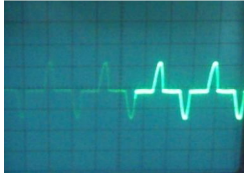
Fig.2: The non-sinusoidal input current wave shape of the supply mains due to rectification action
