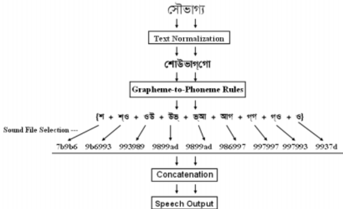
Fig. 4: Diphone selection and labeling process in TTS system
