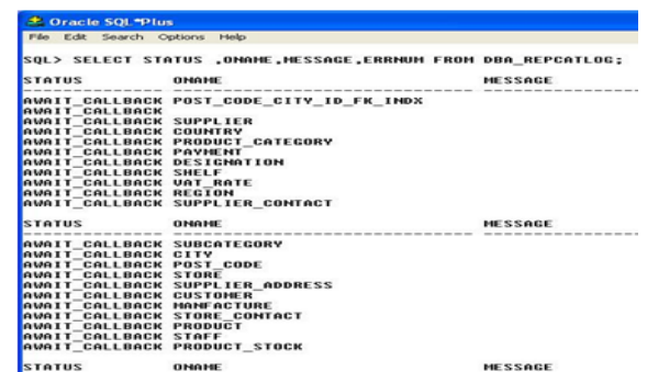
Figure7: Partial output that showing the status of the object in the DBA_REPCATLOG
