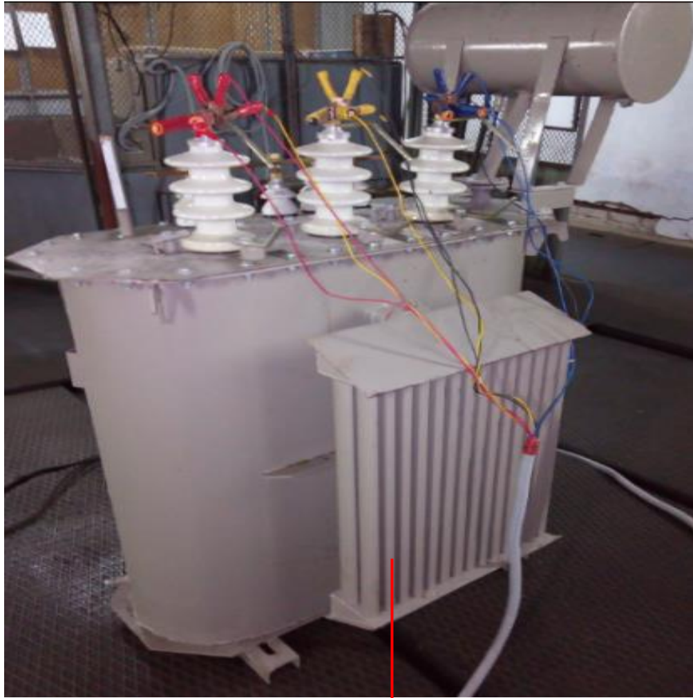
Figure 4.1 200 kVA, 11 kV transformer of conventional radiator under heat run test
