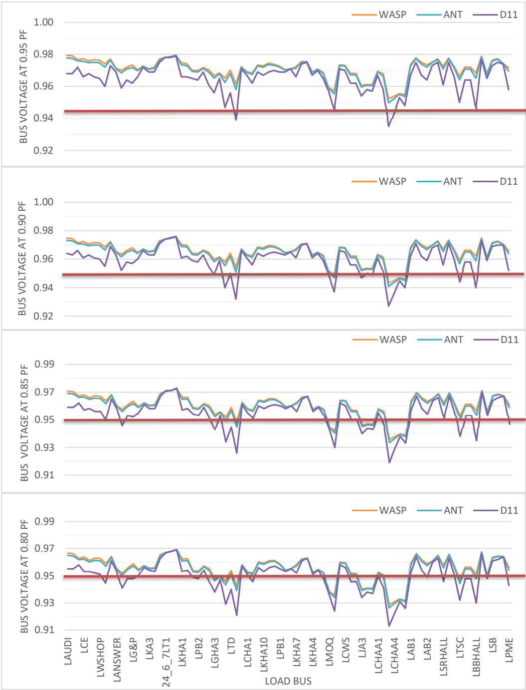
Fig. 4.24. Comparison of L-N Per Unit Voltage at Different PF for Different Cable for Case#4.
