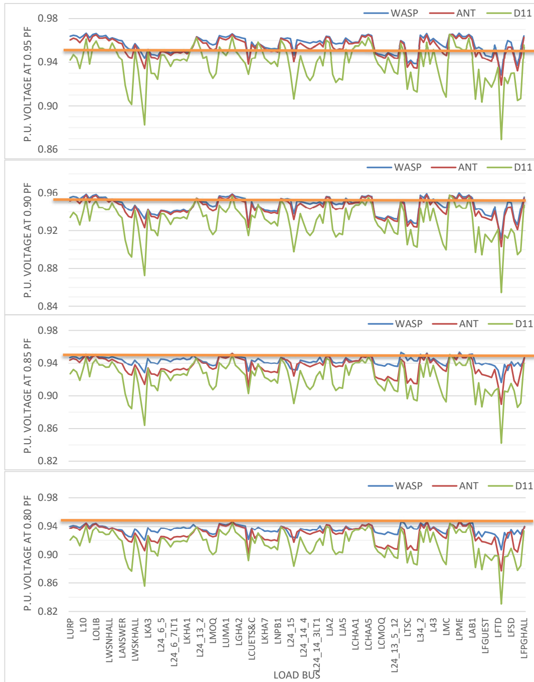
Fig. 4.35. Comparison of L-N p.u. voltage at Different PF for Different Cable for Horizontal Load Extension Model.
