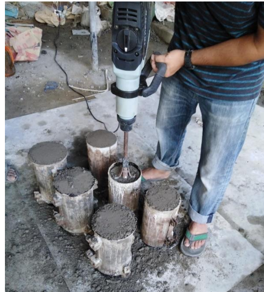
Fig. 3.8 RCC mixture compaction in cylinder
