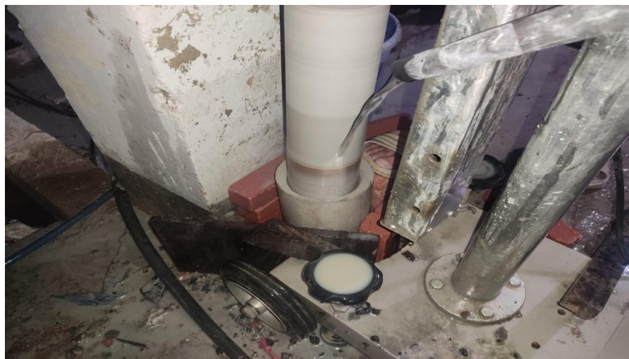
Fig. 3.14: Core Cutting Process
