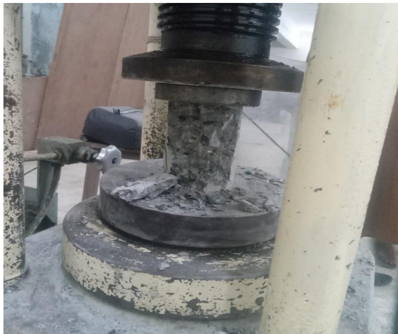
Fig. 3.20: Compressive Strength Test Performed of Core Concrete Cylinder
