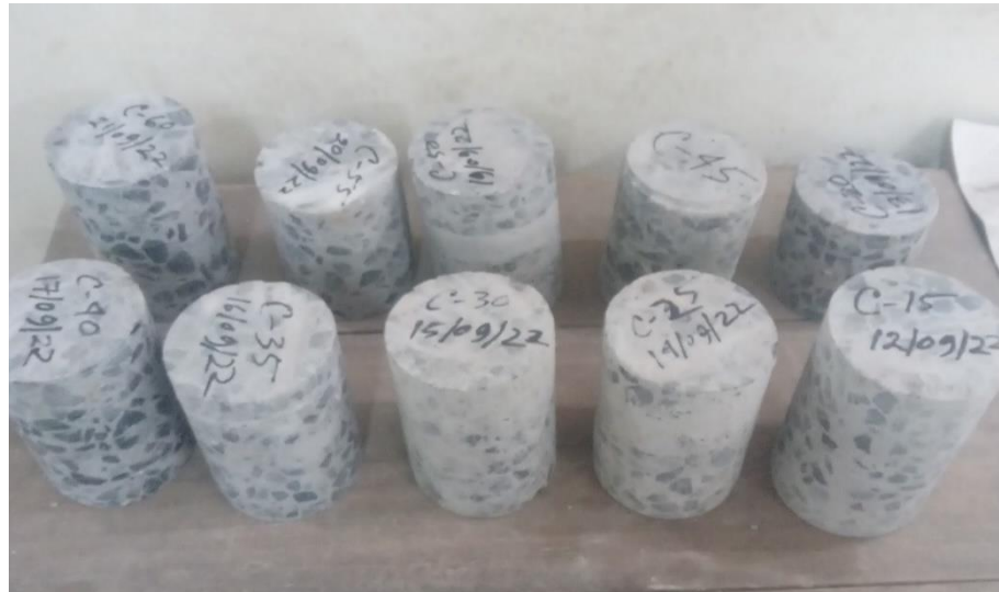
Fig. 3.16: Core Sample after Core Cutting Performed
