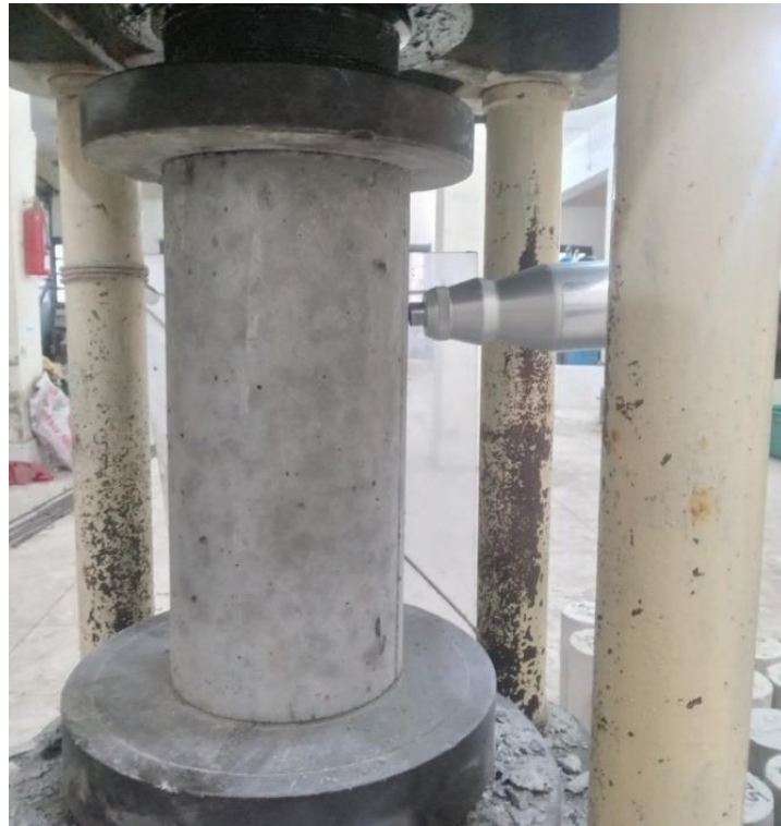
Fig. 3.10: Rebound Hammer Test Performed overCylinder
