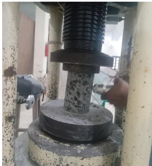
Fig. 3.11: Rebound Hammer Test Performed overCore Cylinder
