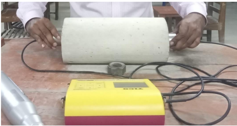
Fig. 3.12: Ultrasonic Pulse Velocity (UPV) Test Performed over Cylinder
