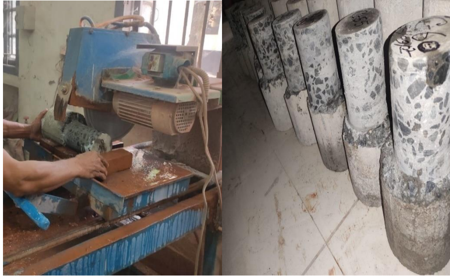
Fig. 3.15: Finishing the Surface of Core Cutting
