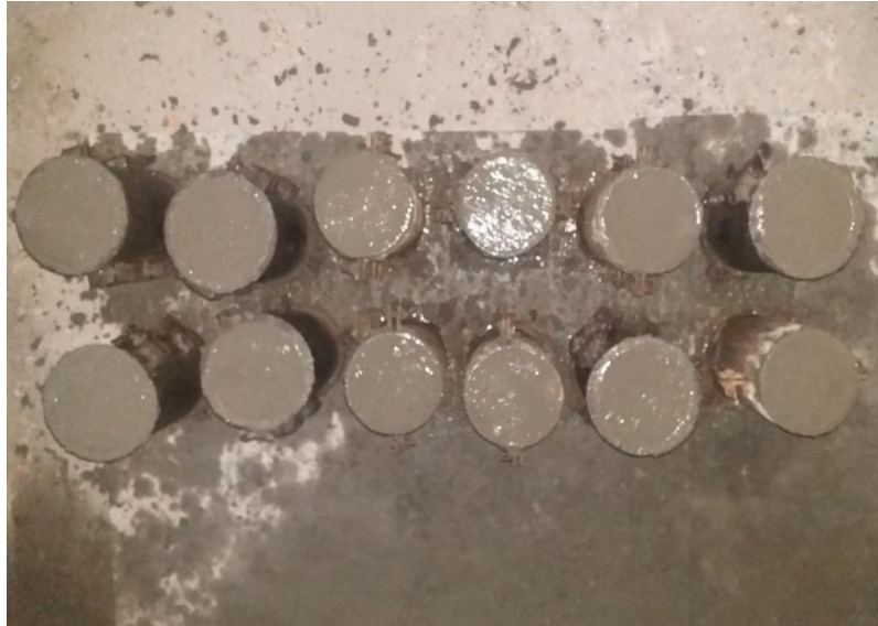
Fig. 3.6: Casting of Concrete Cylinders
