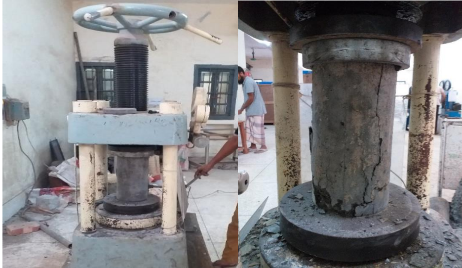
Fig. 3.18: Compressive Strength Test Performance of Concrete Cylinder The compressive strength test performance of Concrete Core Cylinder is shown in Fig. 3.20 . When the test is properly conducted, a maximum load is obtained at the point at which the sample ruptures.
