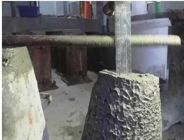
Fig. 3.5: Slump Test of Fresh Concrete
