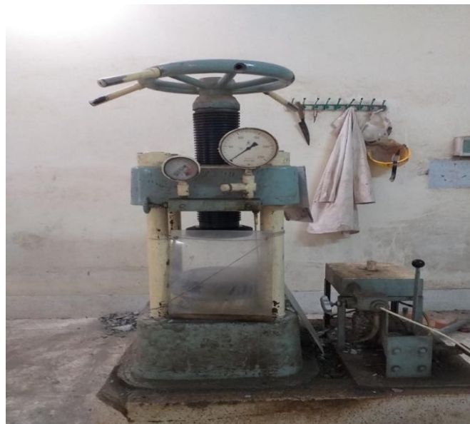
Fig. 3.17: Specimen under Compressive Strength Testing Machine
