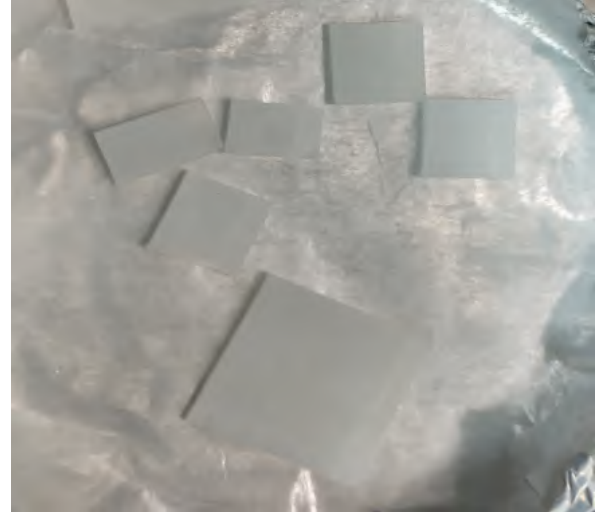
(b) ZnS thin film deposited by SILAR
