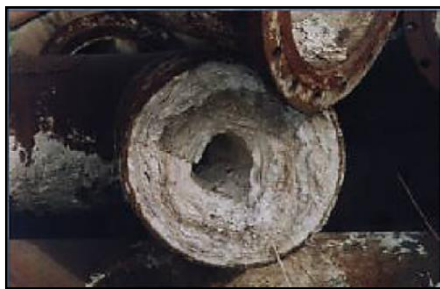
Figure 2.5: Scaling of the Interior Pipe of LPG Recovery Process [54].
