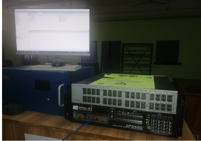
Fig. 4: RT SIL setup with Ethernet cable, host PC, and OP5600 target.
