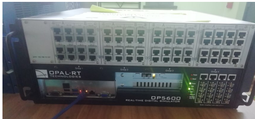
Fig. 2: Configuration of the OPAL-RT Simulator (OP5600).
