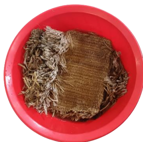
Figure 3.6: Fiber mats are soaked in 5% alkali solution
