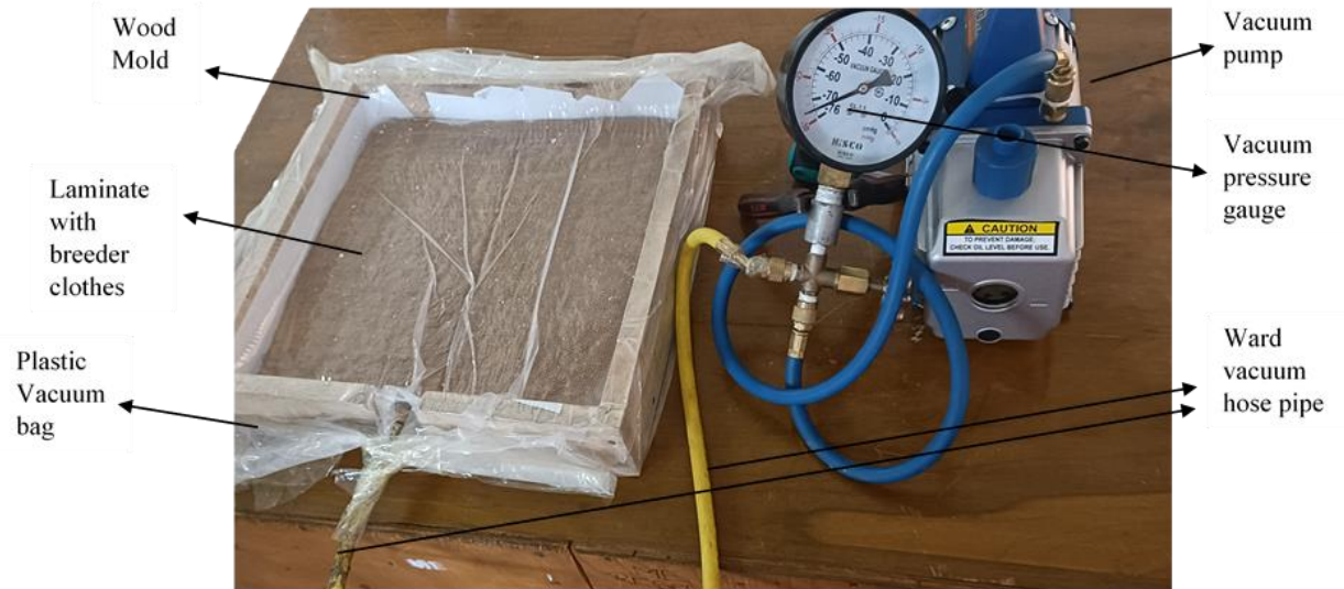
Figure 3.9: Vacuum bag molding setup
