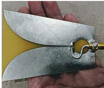
Fig. 3.17. The photo is of fabricated Vivaldi antenna. [56]
