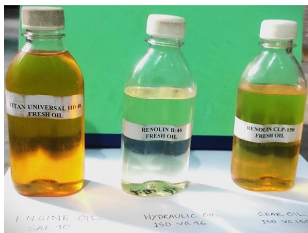
Figure 3.8 Sample of Engine Oil SAE 40, Hydraulic Oil VG 46 & Gear Oil ISO VG 150.
