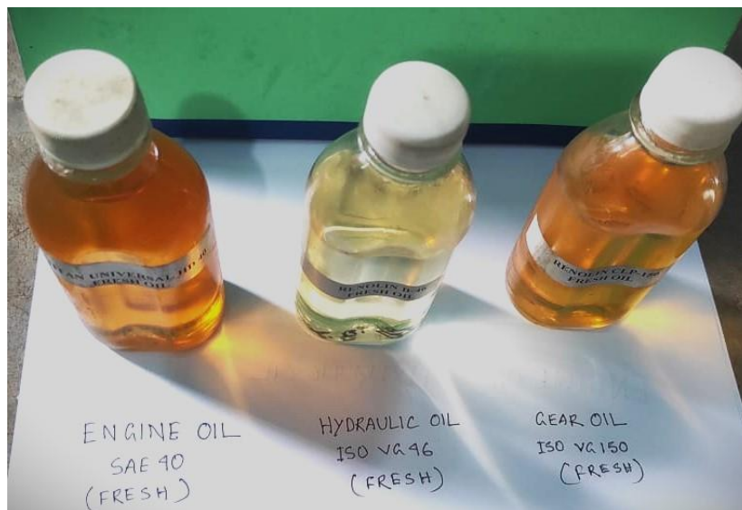
Figure 4.7 Sample of Fresh Engine Oil SAE 40, Hydraulic Oil ISO VG 46 & Gear Oil ISO VG 150.
