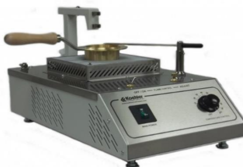
Figure 3.14 Koehler Cleveland Open Cup Flash Point Tester
