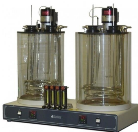
Figure 3.17 Koehler D892 and D6082 Dual Twin Foaming Characteristics Test Apparatus
