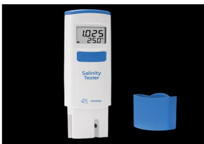
Figure 3.6 Digital Salinity meter
