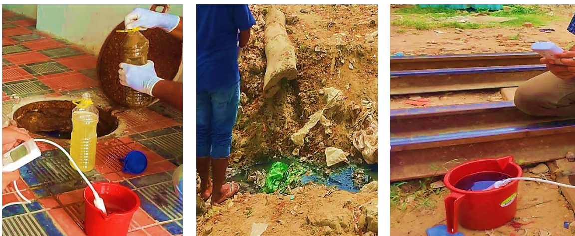
Fig. 3.9 Sample collection and on-spot parameter determination
