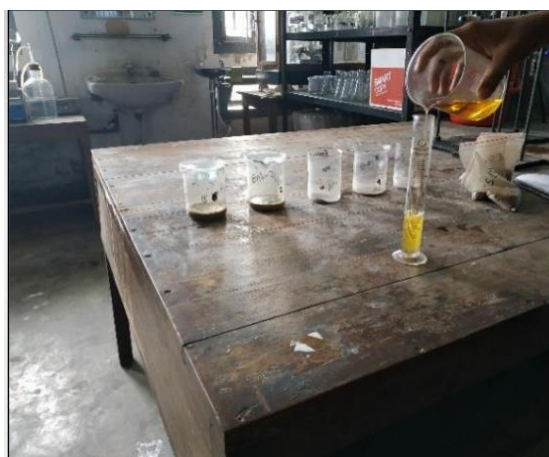
Acid digestion process
