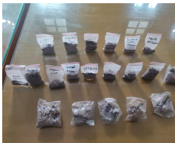
Samples after Sieving and Drying
