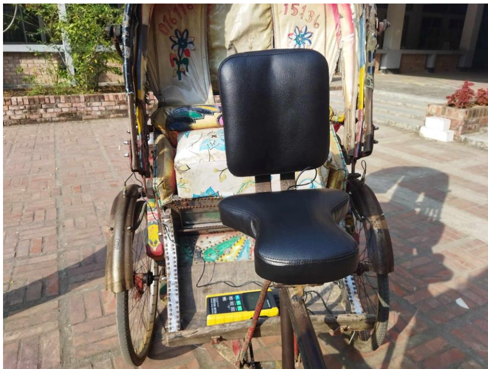
Fig. 3. 6: Rickshaw with fabricated modified seat model
