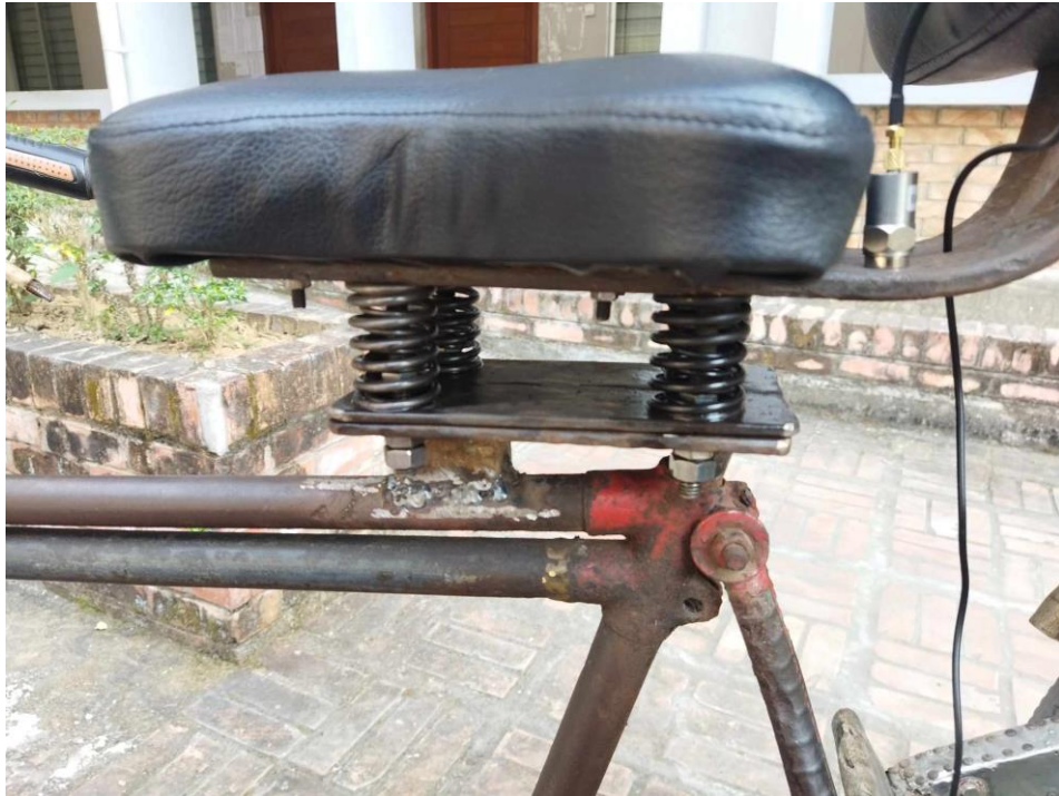
Fig. 5. 4: Vibration meter sensor placed for output data
