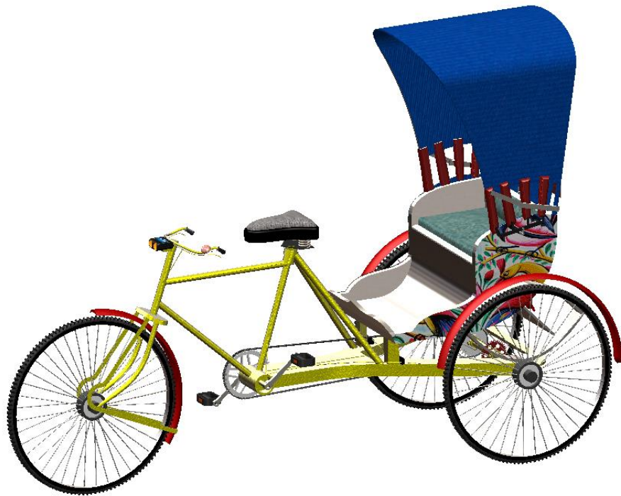
Fig. 3. 4: CAD design of a human powered rickshaw with a conventional seat design.
