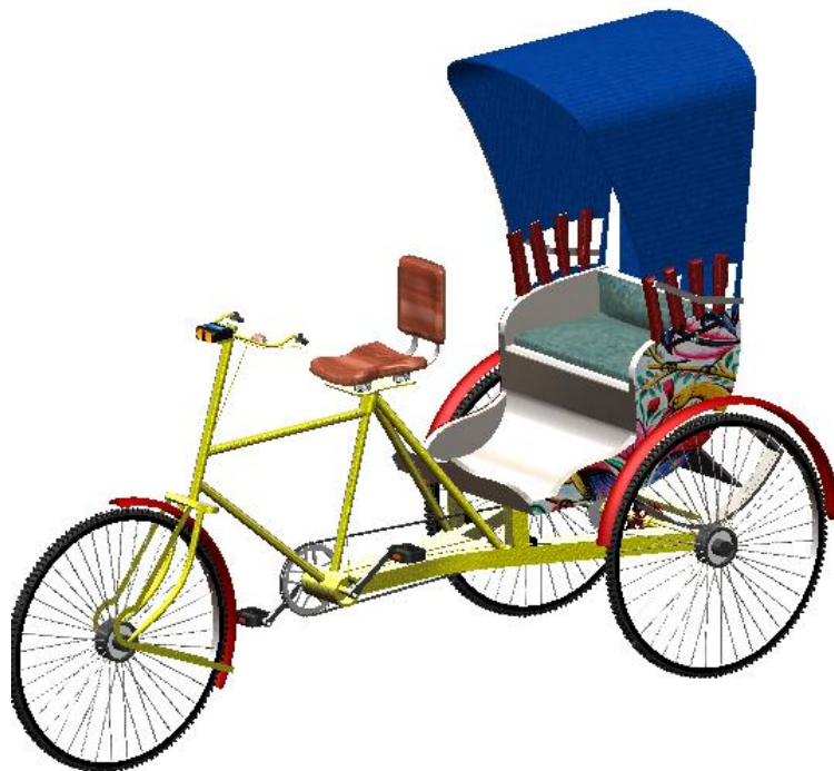
Fig. 3. 5: CAD design of a human powered rickshaw with a modified seat design.
