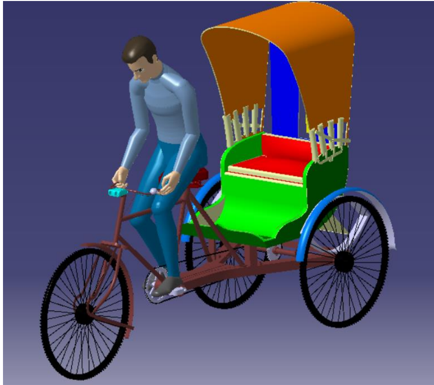
Fig. 4. 1: Ergonomics analysis of human-powered rickshaw with a conventional seat design
