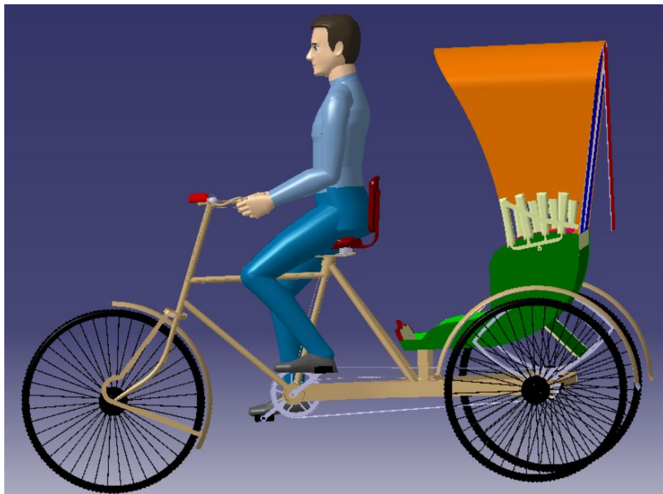
Fig. 4. 7: Ergonomic analysis of Human powered rickshaw with a modified seat design model II
