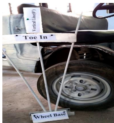
Figure 3.3 Toe-in and toe-out [178].
