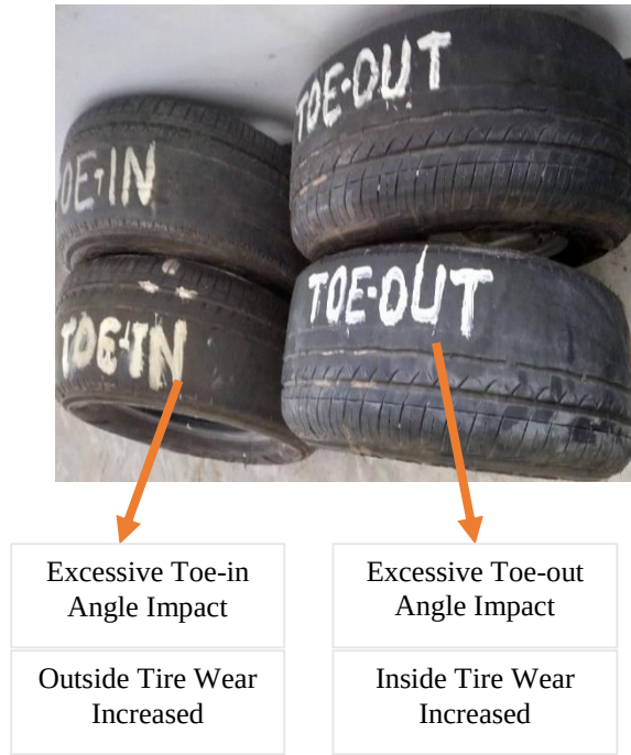
Figure 5.32 A photographic view of tire wear at front wheel total toe-in angle ( 4.20^\circ ) (left) and at front wheel total toe-out angle ( -4.20^\circ ) (right).
