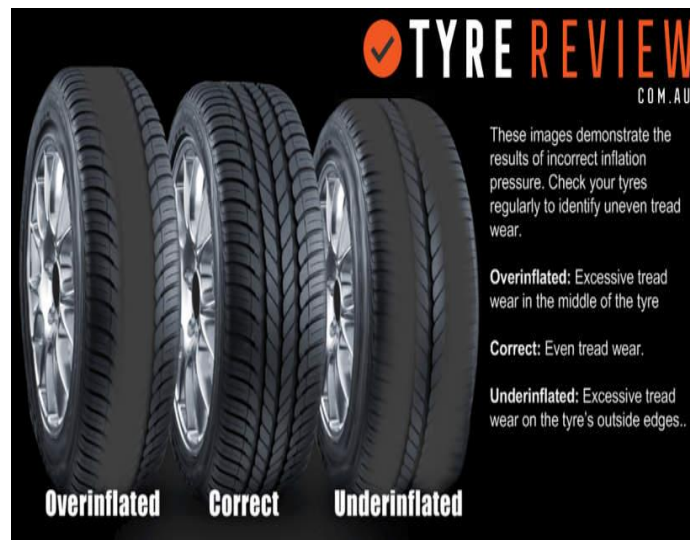
Figure 1.3 Inflation pressure of tire [47].
