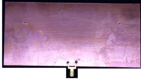
Figure 3.4-1: Fabricated prototype of the presented 5.8-GHz dual-beam switchable single-feed antenna array. (i) Top view. (ii) Bottom view.
