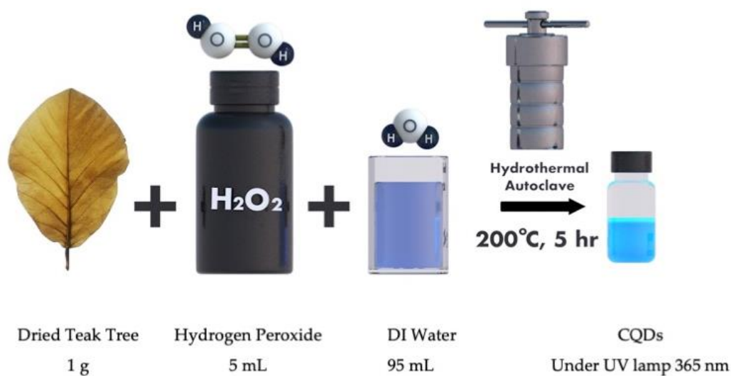
Scheme 3.2: Schematic illustration and synthesis procedure of CQDs.
