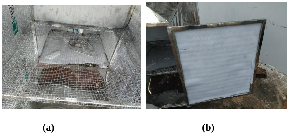
Figure3.3: (a)Drying chamber (b) Thermocol Insulation
