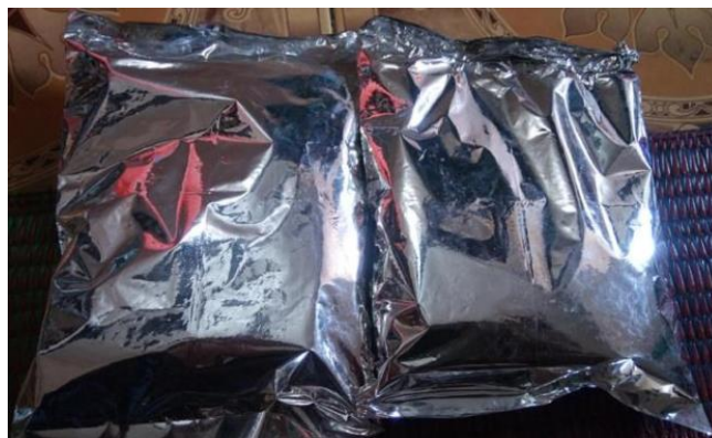
Figure3.4: PCM filled in Aluminum Coated Cover.
