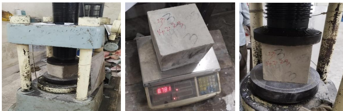
Figure 4.4: Compressive strength test setup in the lab
