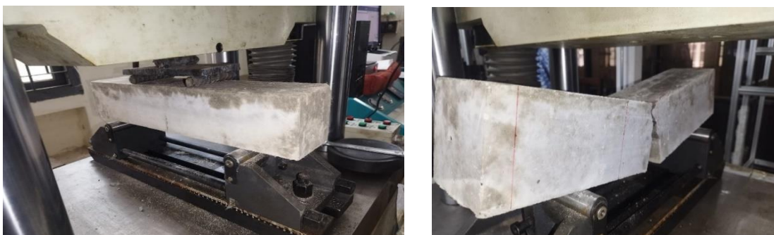
Figure 4.7: Test of fracture energy by Digital UTM
