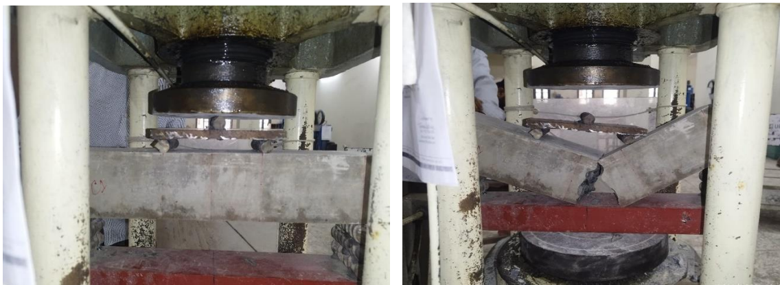
Figure 4.6: Test of Flexural strength of beam in the lab
