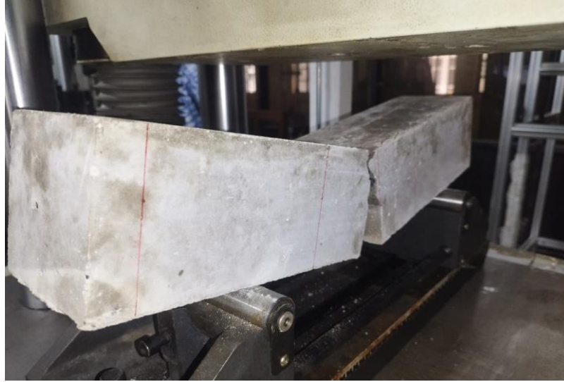
Figure 5.14: Failure profile of Sample Mix-1, Mix-2, Mix-4, and Mix-5
