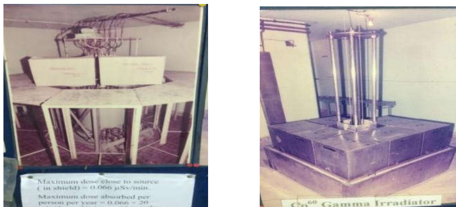
Fig.3.5 Depicts of the ^{60}\text{Co} gamma irradiator setup that was employed in this study.
