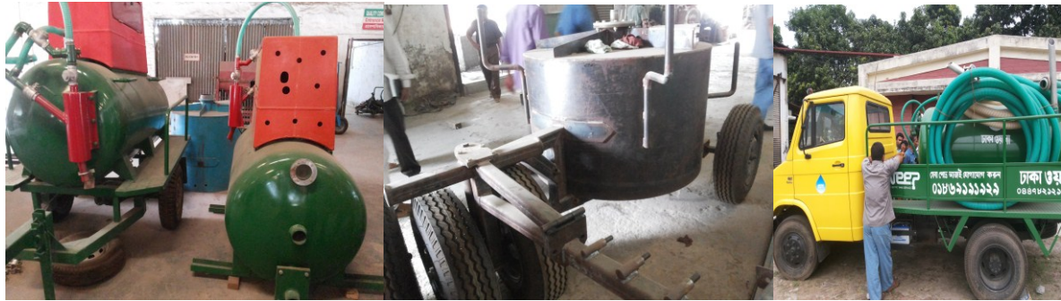
Fig 3: Vacutug MK-VI with Baby Trucks
