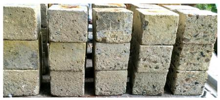
Fig.2 Effect of 3% H<sub>2</sub>SO<sub>4</sub> on 40%, 30%, 20%, 10%, 0% silica powder concrete (left to right)
