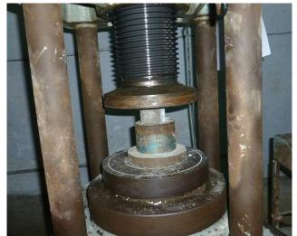
[Fig 2] Mortar Samples is in Universal Testing Machine
