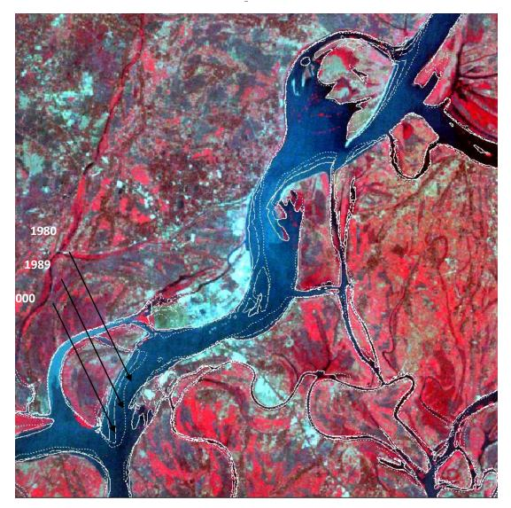
Fig 4 Bank lines from 1980, 1989 and 2000 superimposed on satellite images from 2010. Area covers from downstream of Meghna Ferry Ghat to upstream of Baidder Bazar.
