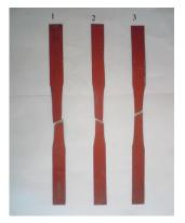
Figure 1: Profiled steel sheet tensile coupon test setup and failure mode
