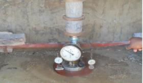
Figure 3. Load test arrangement
