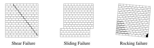
Fig. 2: Failure mechanisms of masonry walls.
