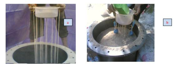
Fig. 4: a) Dry d eposition into calibration chamber from discharging bowl maintaining a constant height of fall, b) Filling of calibration chamber in progress
