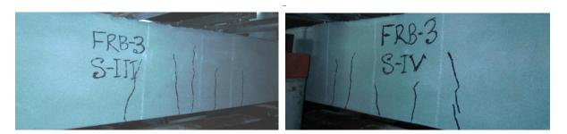
Fig. 4.3: Cracks on retrofitted beams
