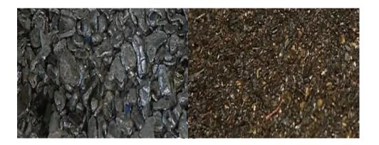
Fig. 7: Aluminum and Copper particles after Recycling (Source: Engineering solution for waste from electrical and electronic equipment)
