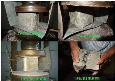
Fig 7: Failure pattern for tensile test
