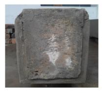
a) Retroffiting of RC beam with wire-mesh in 3 sides b) Retroffited beams (Typical cross-section)
