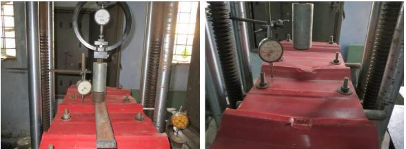
Figure 3: Test setup and failure of mode of web crippling test specimen
