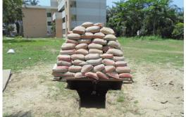
Figure2. Load arrangement for footing load test
