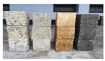
Fig.1 Concrete specimen exposed to 3%, 2%, 1% H<sub>2</sub>SO<sub>4</sub> and plain water (left to right).
