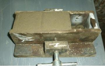
[Fig 1] Cube Mortar Sample Casting
