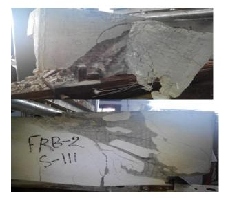
Fig. 4.4: Ultimate failure of retrofitted beams
