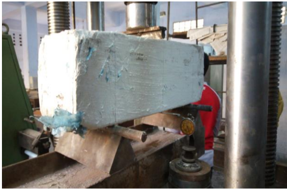
Fig. 5: Flexural test of beam
