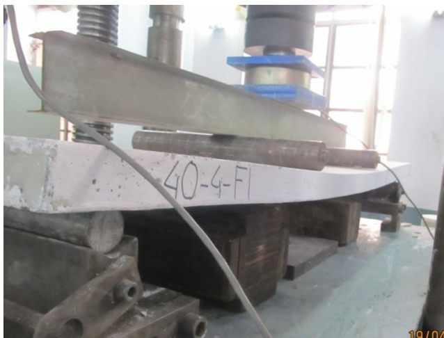
Fig. 1 Test Setup for Flexural Test
