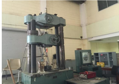
Fig. 3: Test set up for uniaxial testing at Structural Engineering laboratory at AIT
