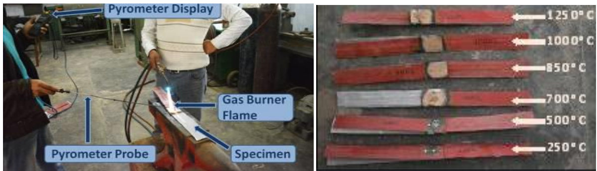
Fig. 6: Specimen at different temperature
