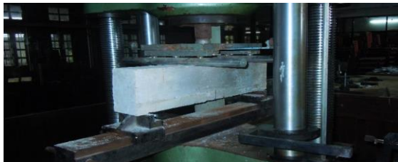
Fig. 3: Experimental setup of crack beam by using brick chips
