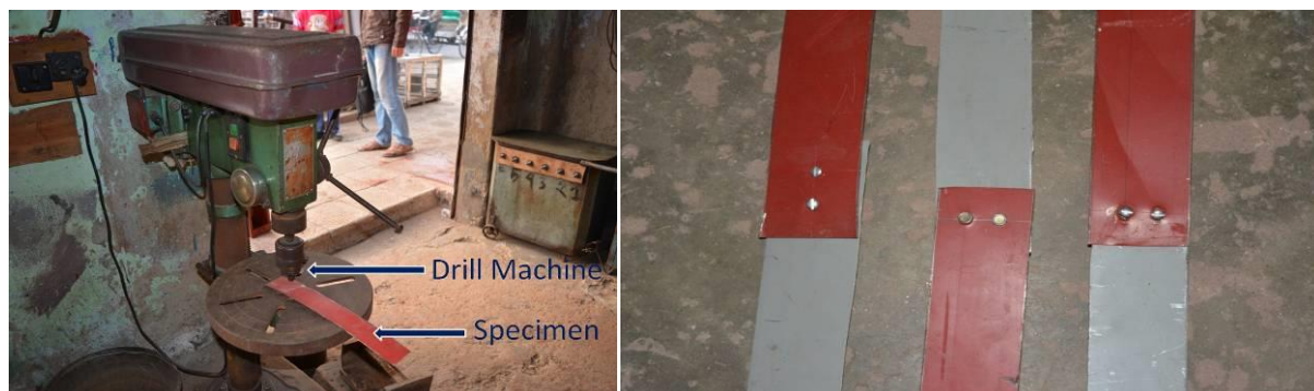
Fig. 4. Drilling and connecting of tensile test specimen
