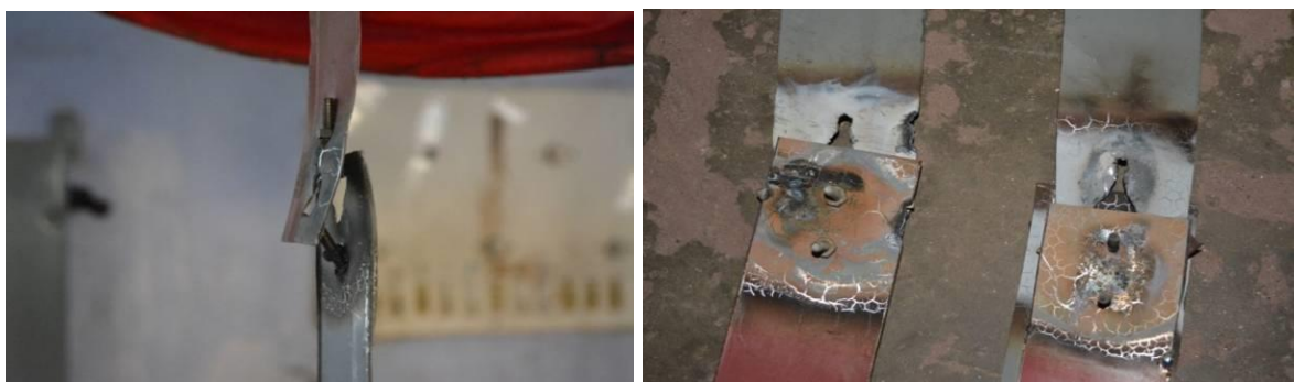
Fig. 8: Bearing failure after elevated temperature
