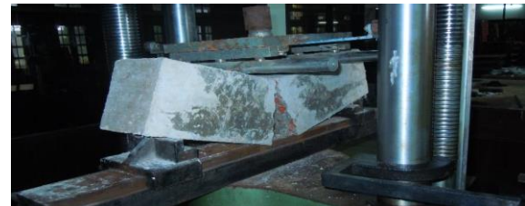
Fig. 6: Failure of uncrack beam by using brick chips
