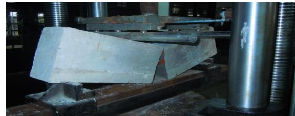
Fig. 4: Failure of crack beam by using brick chips
