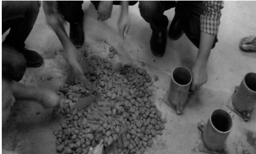
Fig. 1(b): Mixing and casting of cylinders
