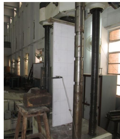
Fig. 2 Test Setup for Compression Test
