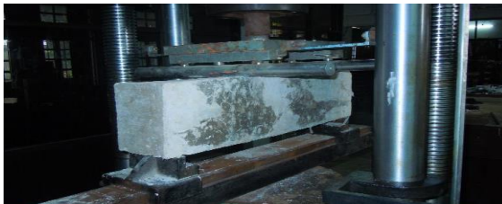
Fig. 5: Experimental setup of uncrack beam by using brick chips
