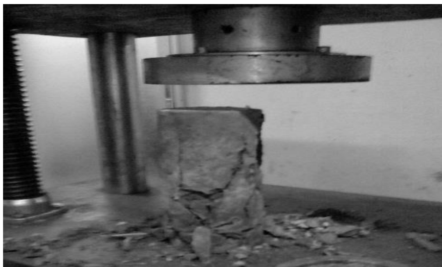
Fig 1(d): Crushing of cylinder
