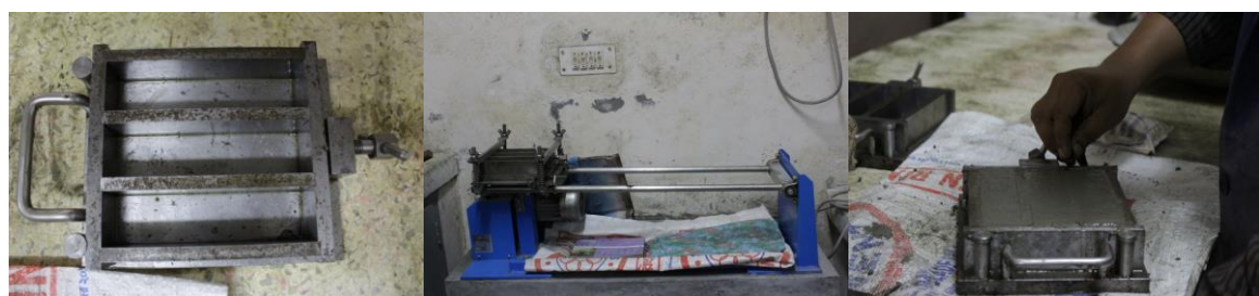
(a) Mould for compressive strength test (b) Jolting apparatus for compaction (c) BDS EN mortar filled moulds Fig.2: BDS EN standard mould, jolting apparatus for compaction and prepared mortar specimens
