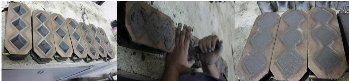
(a) Mould for compressive strength test (b) Hand tamping for compaction (c) ASTM mould with mortar Fig.1: ASTM mould, hand compaction and specimens for compressive strength test of cement
