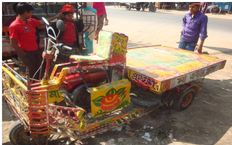
Fig. 2: Motorized flatbed heavy rickshaw or 'vangari'
