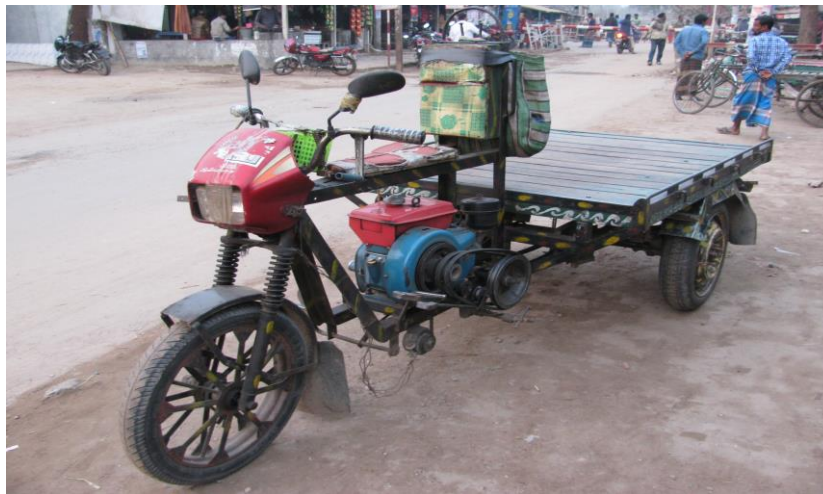
Fig. 1: Motorized rickshaw flatbed with 3 HP Chinese engine
