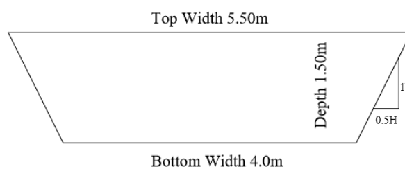
Fig. 2: Existing dimension of canal
